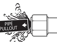
When pipe pullout could occur, pipe joint **MUST** be anchored. Failure to anchor pipe joint could result in escaping line content and cause property damage, serious injury or death.
