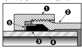
(1) Threaded end-nuts screw onto the threaded body (2), compressing the gaskets (3) against the pipe (4) to make a flexible, bottle-tight seal. The gaskets are confined and protected from damage by retainer rings (5). Note the heavy body construction and ample seating area of the resilient gasket.
