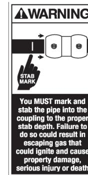
When pipe movement out of the coupling might occur as a result of forces other than that caused by internal line pressure of 150 PSI Max., proper anchorage MUST be provided!
